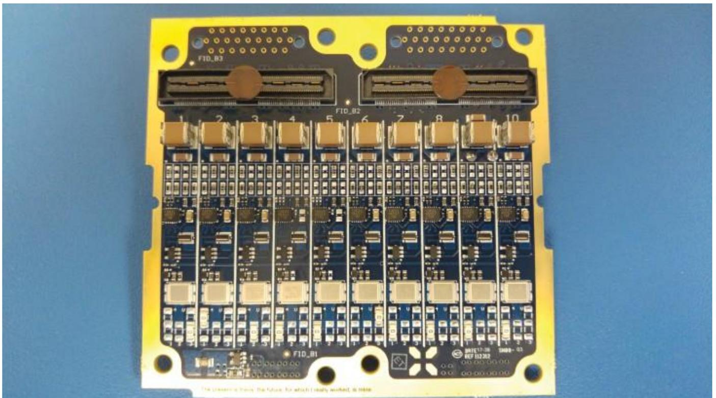
Figure 6: Nova power system peak power trackers
