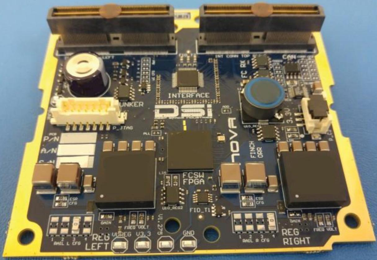
Figure 7: Nova power system scalable power management and distribution systems
