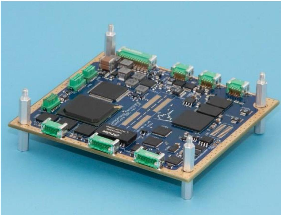
Figure 8: Redundant Explorer onboard computer
