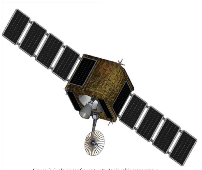
Figure 2: Explorer configured with deployable solar arrays
