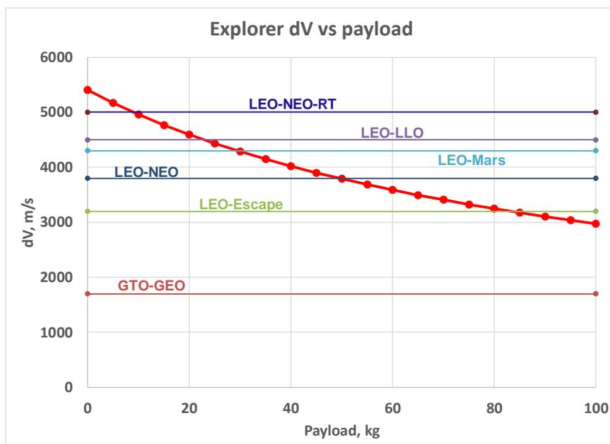
Figure 3: Total delta-V capability vs payload mass allocation along lines of constant mass
