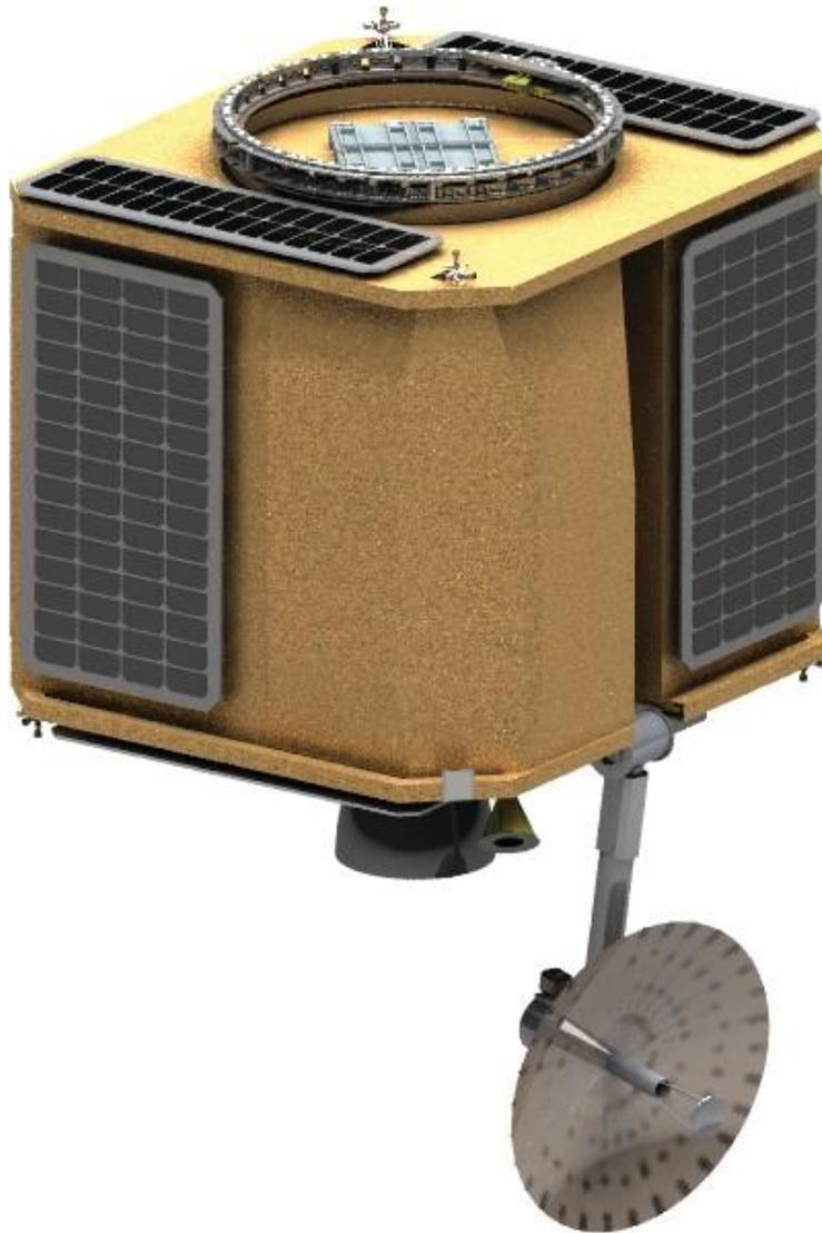
*Figure 4: Explorer configured with body mounted solar arrays*
