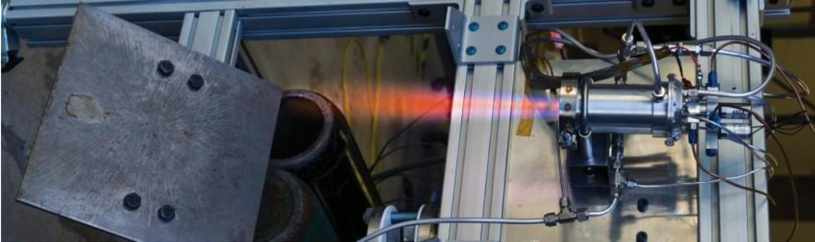
Figure 5: Meteor green bipropellant system under test at Bradford facilities
